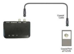
3. Connect another coaxial cable into the coaxial wall port left unconnected in step 1.
